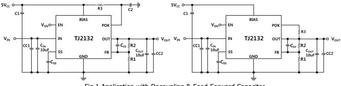
Fig.1 Application with Decoupling & Feed-Forward Capacitor
