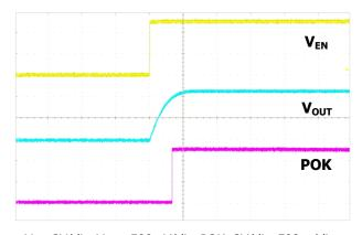
$<sup>\</sup>label{eq:VEN:2V/div, V_{OUT}: 500mV/div, POK: 2V/div, 500us/div} \\ Start up @ I_{OUT}=2A, Circuit ~~\#1 \\ (C_{ff}=10nF, C_{SS}=470pF, R1=R2=10k\Omega, V_{IN}=1.7V, V_{BIAS}=5.0V) \\ \end{array}$
