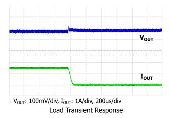
$<sup>(</sup>C_{ff}=10nF, C_{SS}=470pF, R1=R2=10k\Omega, V_{IN}=1.7V, V_{EN}=V_{BIAS}=5.0V)$
